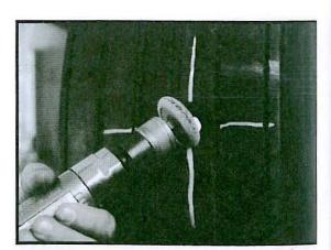
Next, with the appropriate size coarse grit round faced I a Low R.P.M. Air Buffer, remove any excess rubber and rubber from the 45° area of the skive. If necessary, folk with the medium rasp or equivalent to prepare the 45° the skive to an RMA #3 buffed texture.
