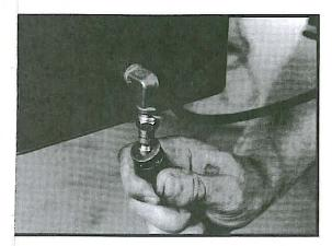
After the allotted cure time, remove the spotter by releasing the air pressure and loosening the hand wheel.
